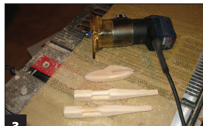
3 Round the pieces. Round the horizontal stabilizer with sandpaper to avoid weakening the tail. Position the other pieces on a non-slip carpet runner and round them with a laminate cutter with a 1/4"-radius round-over bit. The tool's roller bearing will slip into the hole for the wing and produce a contour on the engine booms. This effect was not intentional, but it works well.
