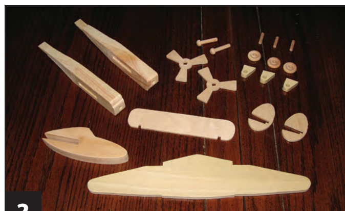
2 Cut the pieces. Use extra care when cutting the engine booms; cut the holes for the wings first. Use compound-cutting techniques to cut the top of the boom. Tape the cut pieces back in place and cut the side profile. Be sure to mark the left and right engine booms; they are mirror images of each other.
